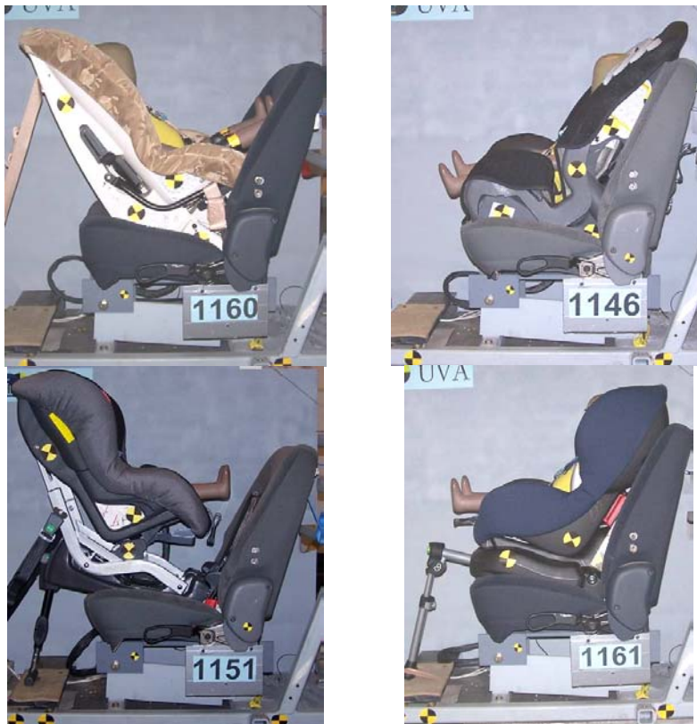
Figure 3 – Pre-test photos of restraints: US2 (top left), US3 (top right), EURO2 (bottom left), EURO3 (bottom right).
