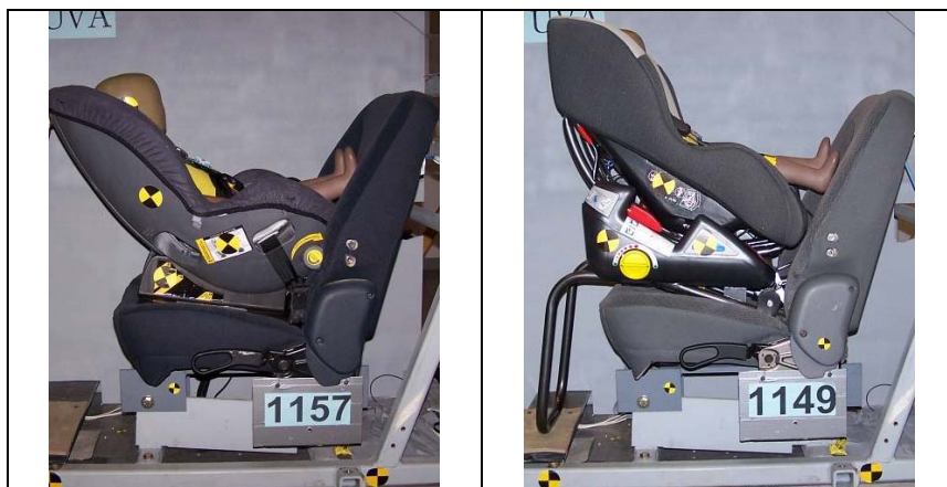
Figure 1 – Pictures of a RF US design with flexible lower webbing (US1, left), and a RF European design with rigid ISOFIX connectors and support leg (EURO1, right).
