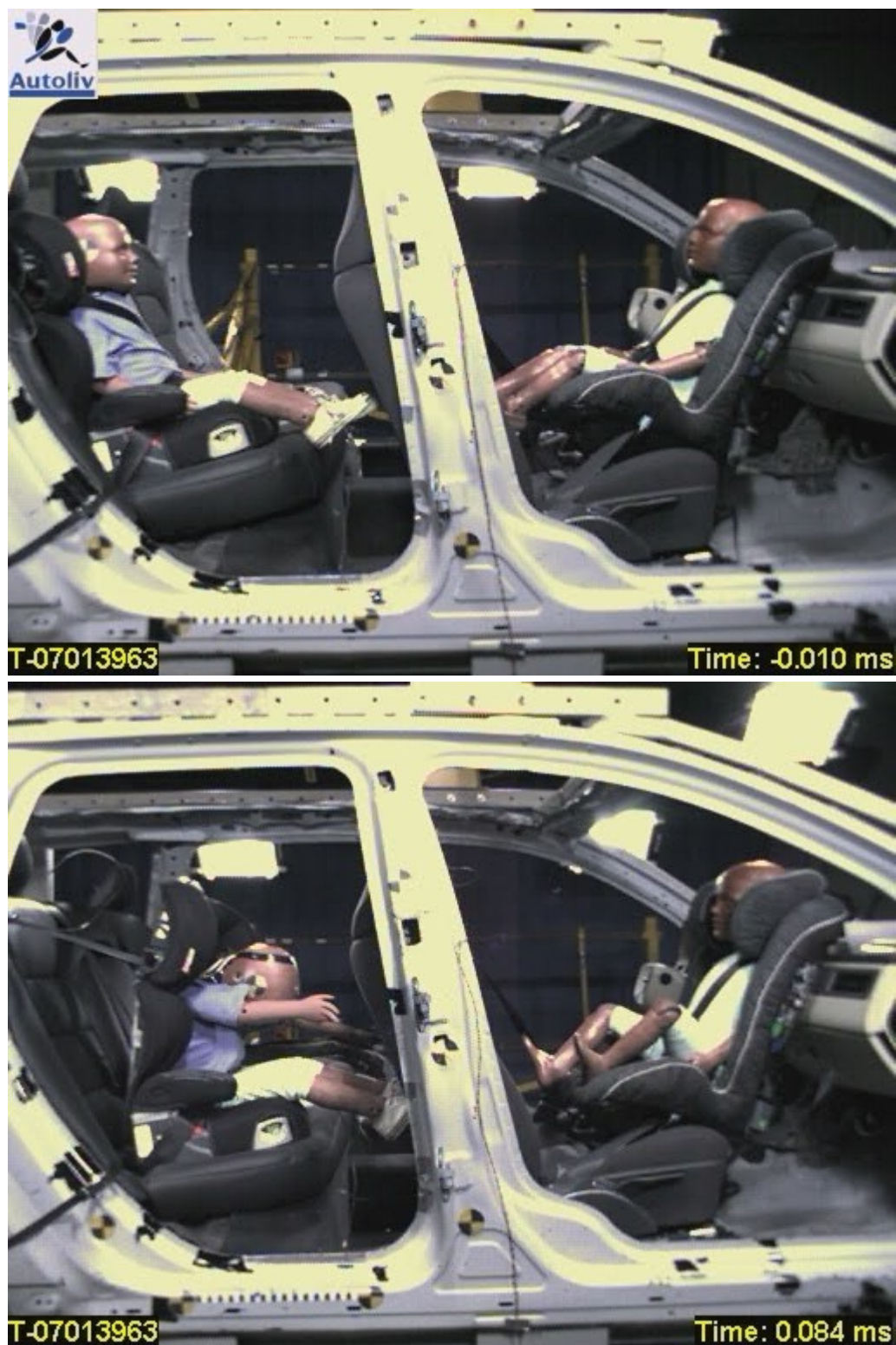
Figure 3 Above picture shows the time 0 ms and the second picture the time for maximum head excursion for the forward facing dummy (at 84 ms).
