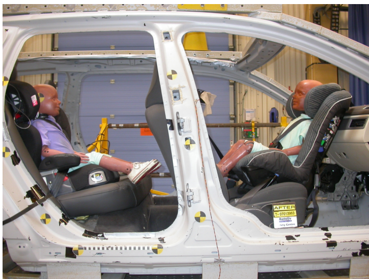
Figure 1 The test set up in the body in white.
